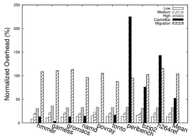
Figure 7: Performance comparison between CREASE and other state-of-the-art approaches using SPEC CPU 2006 when enabling protection
