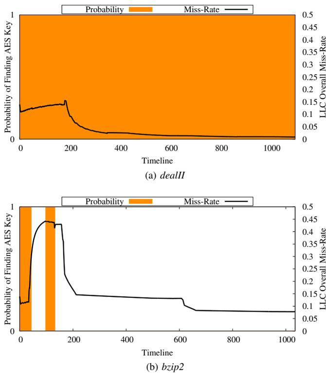
Fig. 5: AES key search trace showing the outcome of the key search and the cumulative LLC miss rate information for (a) *dealII* and (b) *bzip2* benchmarks running on systems without ARM’s cryptographic acceleration support (NoNEON).
